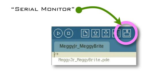
To make your Meggy output serial data, first add the line Serial.begin(baud rate), to the setup section of your sketch.
