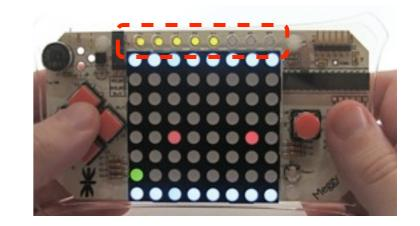
Each LED represents a binary bit, the corresponding decimal values are shown here. The rightmost LED is the most significant bit, with value 128.
